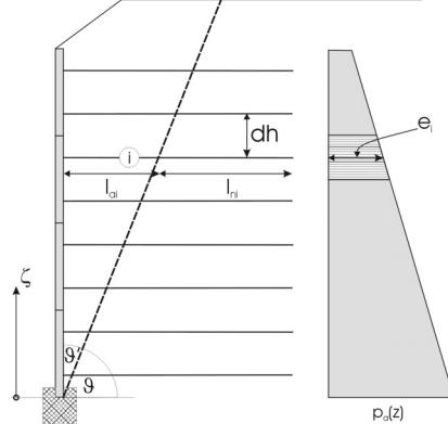
$$\theta = 45^\circ + \varphi/2, \theta' = 45^\circ - \varphi/2,$$
